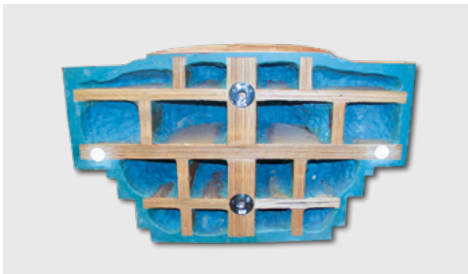
Back of pattern made with OH 11 with PS 03-1
