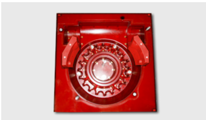
Core box made with GM 984-1
