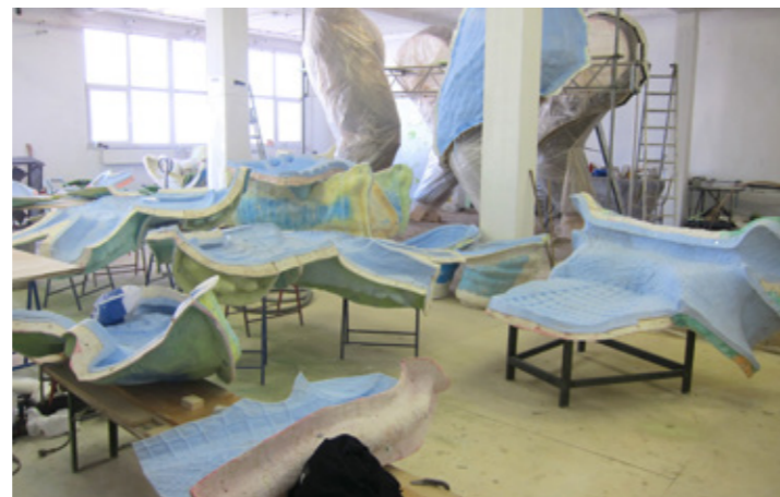
ebacryl production moulds for the dragon skin, which was made of ebalta epoxy resin AH 140
