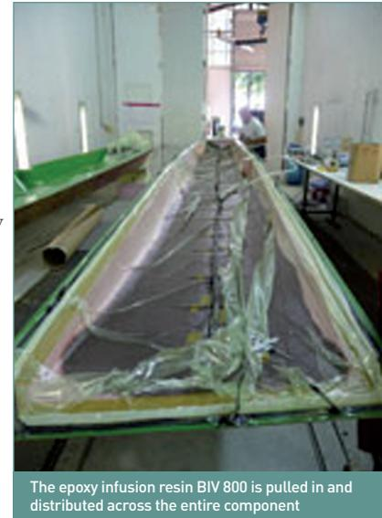
The epoxy infusion resin BIV 800 is pulled in and distributed across the entire component
