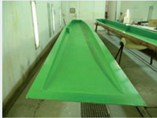
Epoxy mould produced using the vacuum infusion method
