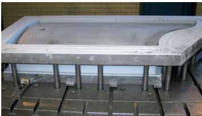
Sheet metal forming tool of eblock® W (outside door layer of a luxury sedan)
