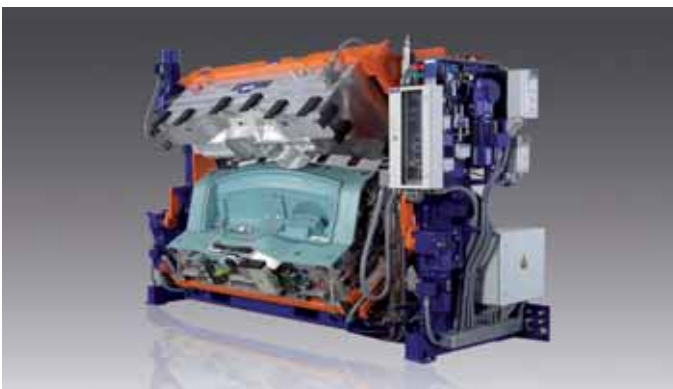
Foam mould of GH 781 Picture credits: Frimo Group GmbH
