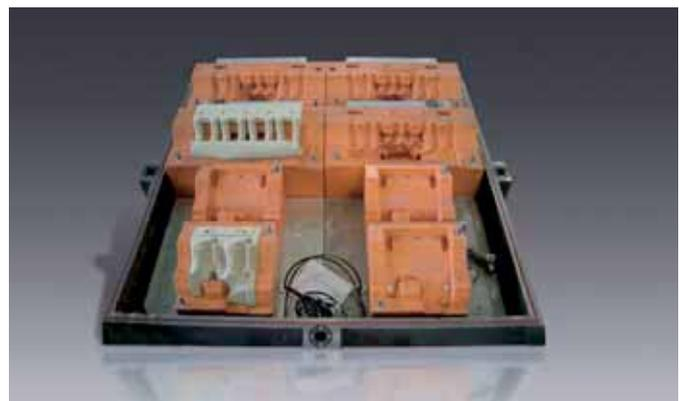
8-fold core box made of **ebablock® K** with core nests
